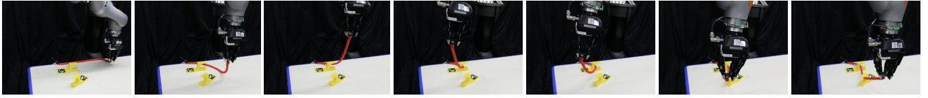
Fig. 5: Physical demonstration with a 7-DoF Kuka arm on cable routing with 3 different cables for a total of 10 runs. Videos are available on our website.
